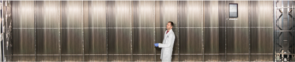
Neutron experiments require large areas of neutron detectors, such as this 40-square-metre detector for neutron spectroscopy. © STFC
